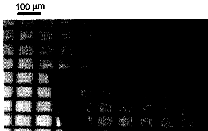
FIGURE 10 — Optical micrograph of a Microcup ® EPD showing partially addressed Microcups ® using a sharp-edged electrode pattern.
